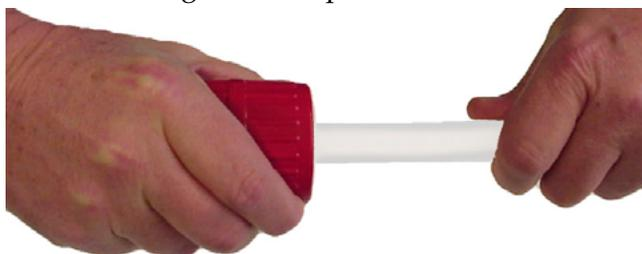
*LK PE-X Universal Pipe can be deburred using the same type of pipe reamer used on copper pipes.*
