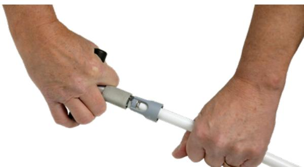
*LK PAL Universal Pipes must be calibrated and deburred using an LK PressPex Calibration Tool F9.*
