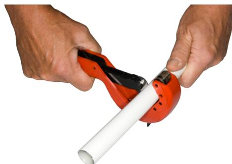
Cutting done with a pipe cutter fitted with plastic fitted with cutting wheels for plastic pipes.
