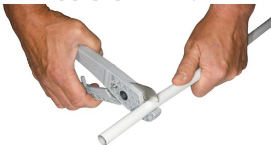
*Cutting performed with a pipe cutter.*
