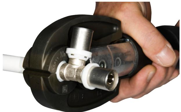
Any gap at the front of the jaws may be due to solid residue between the jaws; this will prevent proper compression.
