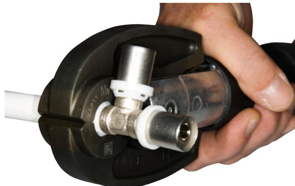
Any gap at the front of the jaws may be due to solid residue between the jaws; this will prevent proper compression.
