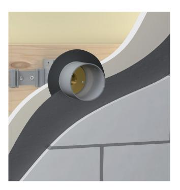
14. If the wall cladding is of ceramic tiles, the pipe membrane should be assembled behind the tiles and connected tightly against the wall lead-through. **LK Pipe Membrane Wallbox Push**, (Article no. 481 44 23) can be used. The sealing layer contractor is responsible for the sealing layer's adhesive properties in accordance with the industry rules.
