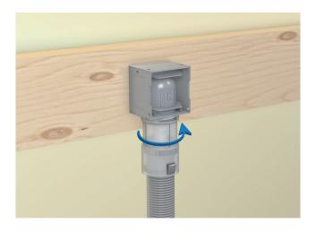
12. Assemble the sleeve coupling on the wallbox's casing with a rotating movement until it stops, so that it locks firmly. Then pull the conduit to ensure that it is secured firmly in the sleeve coupling's lock clips.
