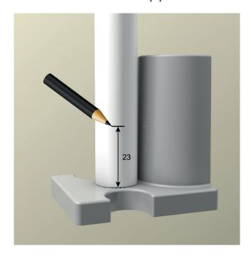
5. Mark the insertion depth on the PE-X pipe. The insertion depth should be 23 mm on the 16 mm pipe and 27 mm on the 20 mm pipe. The yard-stick at **LK SmartTool** (Article no 188 07 41) will facilitate it.
