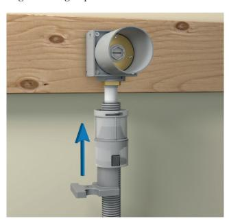
11. Use tool **LK SmartTool** (Article no 188 07 41) to push the sleeve coupling up outside the 25 conduit to the housing. Use the LK SmartTool as in the picture above so that it opens the lock clip in the sleeve coupling. Alternatively, place a piece of slitted 34 conduit (min. 10 cm long) outside the 25 conduit.
