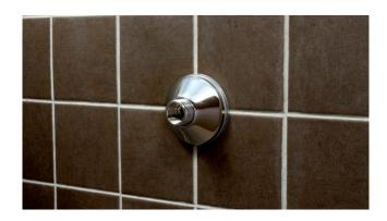
For assembly of tap mixer in accordance with international standards, **LK Connection coupling** 34" 1 12" (Article no. 187 05 46) should be assembled. The length of the connection coupling should be adjusted so that approximately 10 mm of the 34" pipe thread is exposed when the cover plate is tightened against the wall. The thread joint against the angle fitting should be sealed with, for example, flax and thread paste. Thread tape should not be used. Tightening is done with a 14 mm Allen key.
